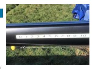
don't get 'block to block' at the boom before you have full kicker. The kicker (like mast rake) is a critical control so it needs to be calibrated to replicate fast settings while racing. There are several ways of doing this, but I like to use calibration stickers on the boom using a string arrangement off the kicker cascade back along the boom with a small bobble as a reference. (see picture right). Mine has a 2:1 'doubler' to make the gauging more accurate (see left picture below).
