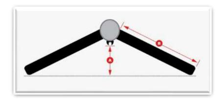
Spreader deflection (distance A) controls how much the mast bends fore and aft. A fuller deflection (with distance A longer) will allow more mast bend, so the sail will be flatter with a more open leech (less power). This may suit lighter sailors who may want a slightly de-tuned rig. A shallower deflection (with spreaders further forward) will give more sail power and is better for heavier sailors.
