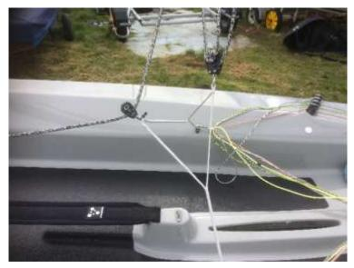
On the Mark 1 boats, the bridle length is nominally 470mm. On Mark 2 boats, it is around 500mm (unless a mini-traveller arrangement is used). It is better to have the bridle too long rather than too short. Getting the correct length makes a significant difference and you can shorten it by 25mm for windy days if you have it adjustable.
