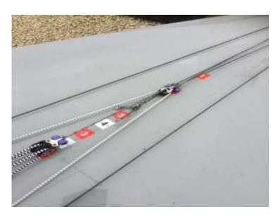
Having the rake calibrated will allow you to repeat rake settings quickly during a race, for example to depower or for pointing higher. The important thing is to have some reference somewhere on your mast rake as this is one of the critical controls – you want to be able to repeat settings without thinking twice about it.
