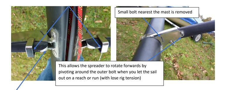
You may have to file down the back corner of the spreaders to make sure they don't catch on the mast or bracket. They are soft aluminium so it's not difficult to do.
