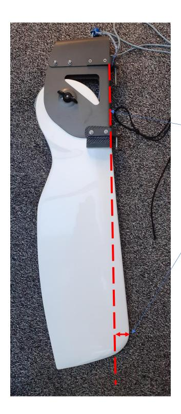
Taking a straight line down the front of the rudder stock and project it down the rudder blade.
