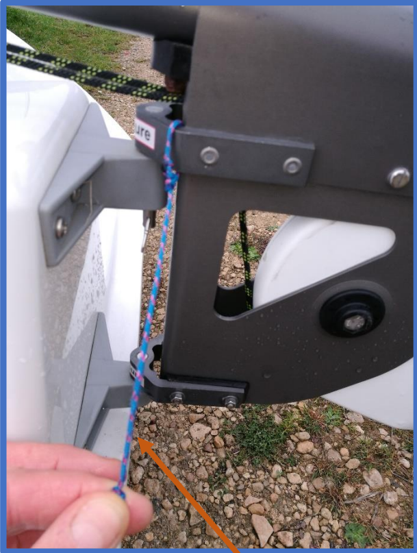
2mm Cord, tied to the top pintle fitting with a stop knot in one end. The end of the cord and stopper knot should come down to the bottom rudder fitting, which should be about the right length.
