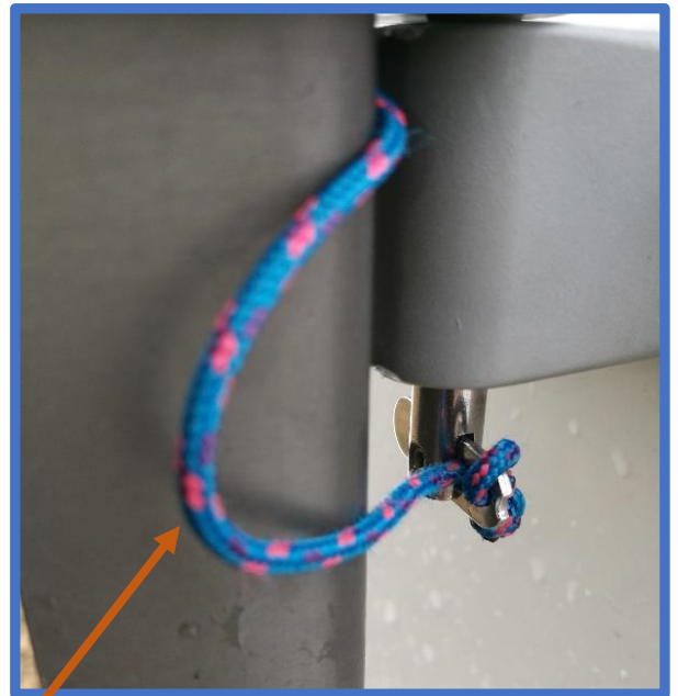
Pull this end to tighten the loop and secure the retainer in place
