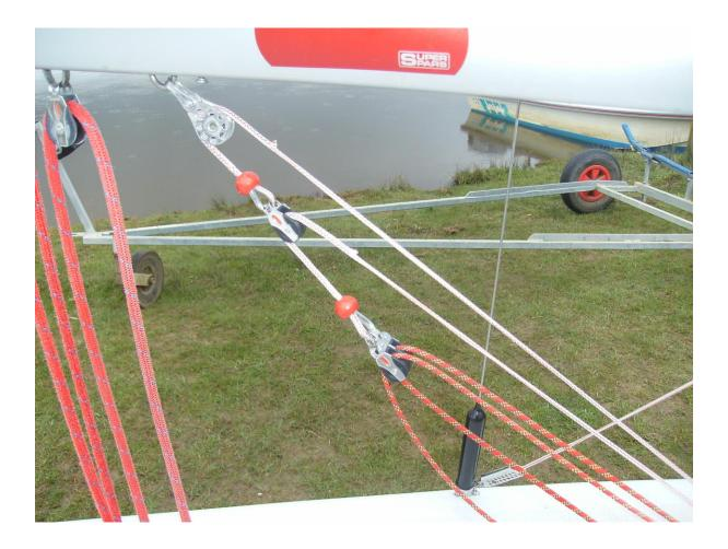
When it gets really light the centre bridle gets in the way of getting right forward. On Richard's Mk1 boat he had a length of thin rope permanently tied to the loop in front of the centre mainsheet block and kept tidy when not in use by a length of elastic.
