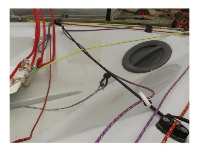
The Mk1s clew was attached to the boom with a slider in a track. This can create quite a bit of friction and makes it difficult to adjust the outhaul whilst sailing. Here some plastic/mica has been attached under clew outhaul pulley to allow it to slide more easily. You can also revise the set as per current Mk2s which have removed the slider altogether and instead simply tie the clew to the boom with a strap/rope (a la Laser style clew strap).
