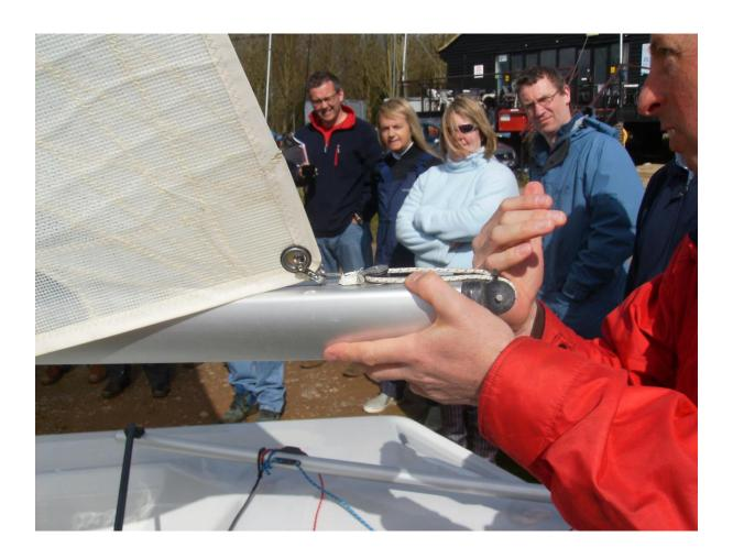
Here the standard multi-block kicker has been replaced with a modern cascade system - again using dyneema. This became the standard kicker system for Hartley built Mk1 boats and is still used today for the MK2e. The advantage of this system is that it allows finer and smoother adjustment. (You may also spot that the lowers have been replaced with dyneema! - to save weight, this is not a standard item but is permitted under the class rules).
