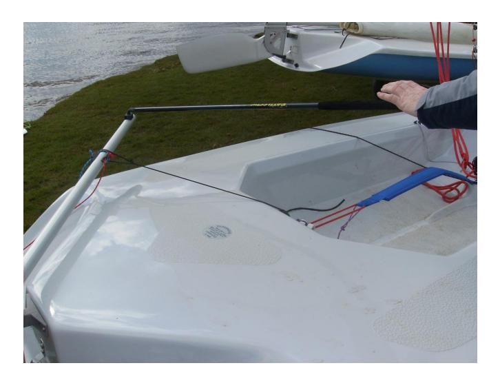
Both the adjustable mast rake and the kicker system are continuous which means that there is no end to the control line. It is a joined-up loop. A 4-5mm Excel Racing line which has a dyneema core. Dyneema d12 if you haven't come across it is very easy to splice. Both of these control lines are long enough so that they can be adjusted whilst fully hiked - and the kicker long enough so it doesn't foul the centreboard.
