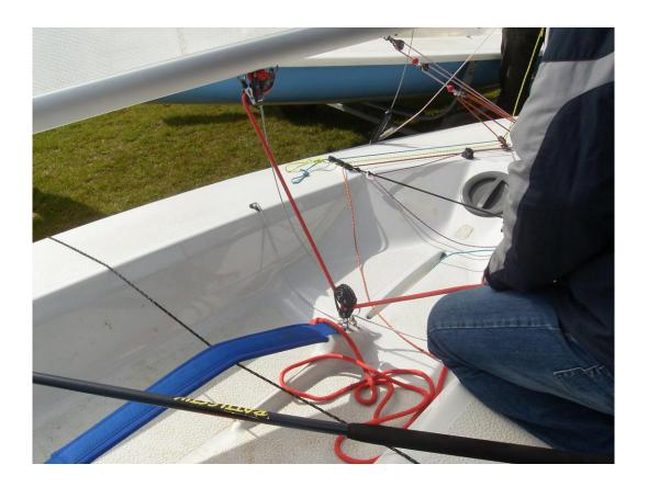
Later Mk1 boats built by Hartleys incorporated a ramp under the mast step from new, earlier boats can retrofit the ramp which was allowed under the class rules in recognition of the amount of mast rake now being used by a lot of the top sailors. Richard has a retro fitted a ramp under his mast step making it from an old chopping block (not wooden!). With ref to V7 of the Class Rules the maximum height of any point of the mast ramp must not be higher than 12mm.
