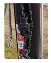
Option 2: Replace the Clamcleat with a small "Mast Hook Rack". This is the most secure system and with a Dyneema rope guarantees that the halyard can't stretch or slip and the mainsail will stay
