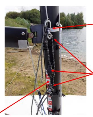
Allen 20mm Block with hook, hooked through the loop that is spliced into the core of the dyneema rope.
