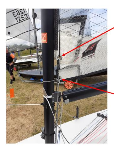
Shock cord is now attached to the mast spreader fitting and runs down through the top eyelet, the same eyelet that the Cunningham control line runs through. As you can see, you now have the shock cord pulling up and the control line pulling down...PERFECT
