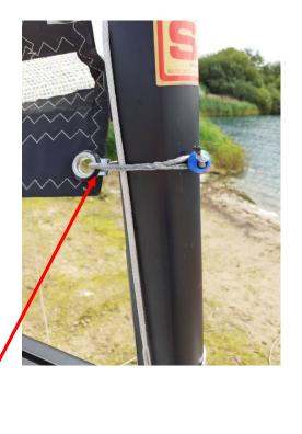
Then make a rope strap that will attach the sail around the mast as shown above, this is the same arrangement as the clew strap that holds the sail to the boom. I used 4mm dyneema, I made a loop in one end and then used a small stopper at the other end that I could pass through the loop to form the strap. The length is important, see note below
