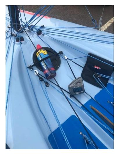
The other addition Mat has made is a control line take away system using bungie to pull the slack from the free end so that the loose ends don't just sit tangled on the floor, again this is personal preference but Matt is such a master rigger I wanted to share it with you so you can see there is plenty you can play with to make the control line arrange fit your personal preferences. Anyway, happy fiddling and thank you to Matt for sharing your latest rigging ideas with us all.
