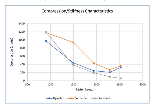
You can see that the standard untapered battens are very soft, especially the bottom two longer battens. This makes the leech quite sensitive to oversheeting and applying too much kicker tension. If you don't get it right you will lose power and not be able to point.
