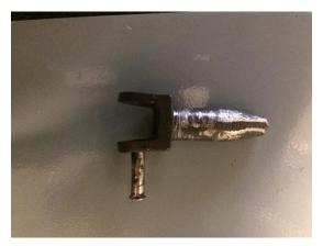
2. Although the aluminium alloy has high tensile strength, it is susceptible to permanent deformation under extreme stress conditions, such as a broach capsize downwind to leeward when the rig hits the water and the momentum of hull and rig subjects the gooseneck to sudden high forces. This has resulted in the gooseneck shearing or breaking away from the boom. In normal use, over time, the pin flanges can permanently distort and the toggle-pin rivet can start to pull away.
