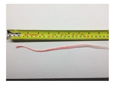
The ends will be a bit ragged, so cut off the ends neatly with Dyneema scissors (see my splicing scissors review). You can cut the ends with the Electrician's scissors (Screwfix Product 96347 £14.50) but they must have good blades. I found that cutting the telltales to 4 or 5 inches is about the right length. If they are too long they will tend to fray at the ends and stick more easily to the sail.
